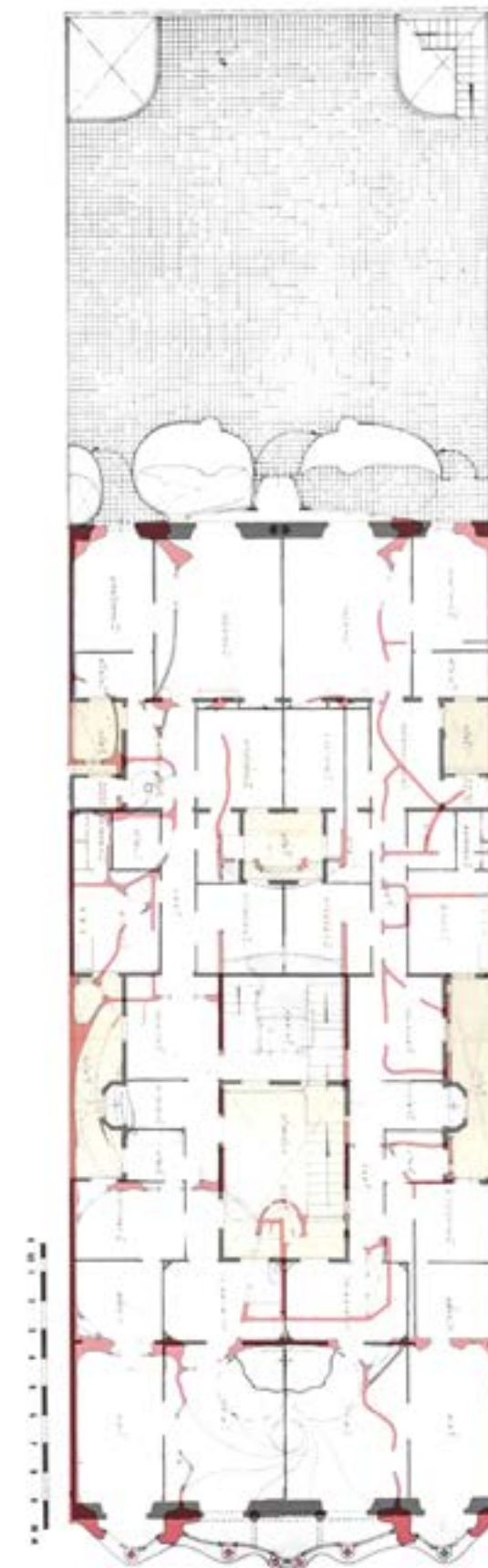
Red: walls and dividers in 1952, Amics de Gaudí. Black: walls and dividers in 1875, Emili Sala's building.
